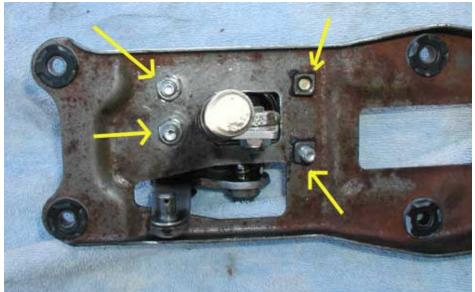
4. Note the position of the lower shift lever pivot with regards to the neutral return spring before removing the lever from the shifter.
