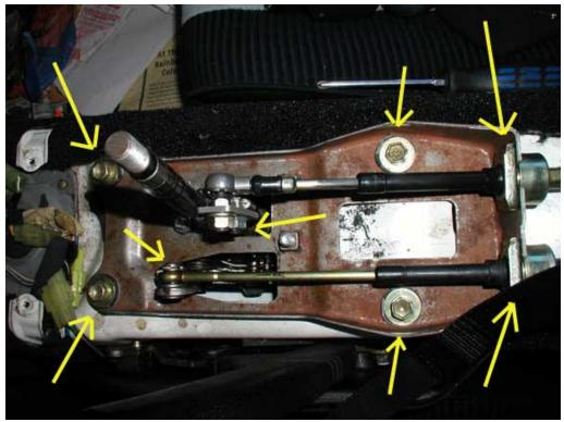
3. With the shifter assembly removed from the vehicle, disassemble it by removing the 4 12mm bolts. Retain one of these bolts and the two nuts.
